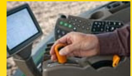
Speed adjusting wheel With an easy to operate thumbwheel, set the maximum forward or reverse speed for each speed band; the Electronic Management System ensures smooth, quick and powerful acceleration or deceleration, regardless of load or ground speed
