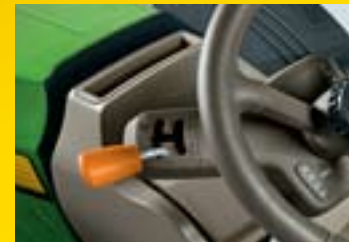
Left-hand reverser Instantly change direction without readjusting your speed (right-hand reverser option also available)
