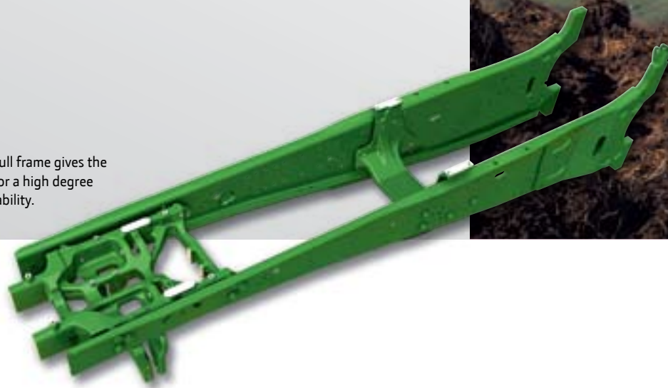
The full frame enables heavy loads to be lifted and transported.
